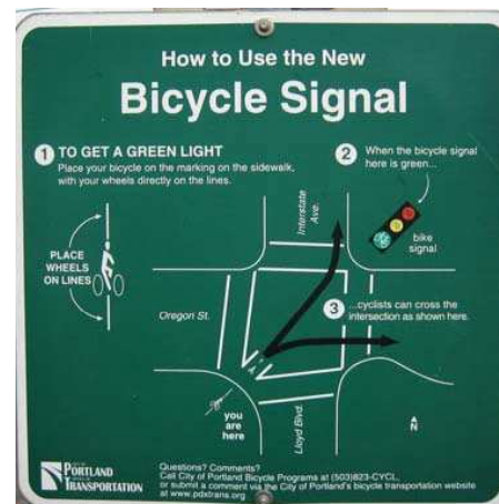
Half-signals for bicyclists should be clearly marked to minimize confusion.
