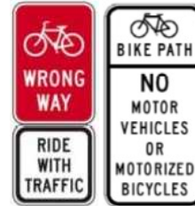
MUTCD Sign R5-1b and R9-3c are regulatory sign. The bicycle path exclusion sign (R44A) is specific to the CA MUTCD.
