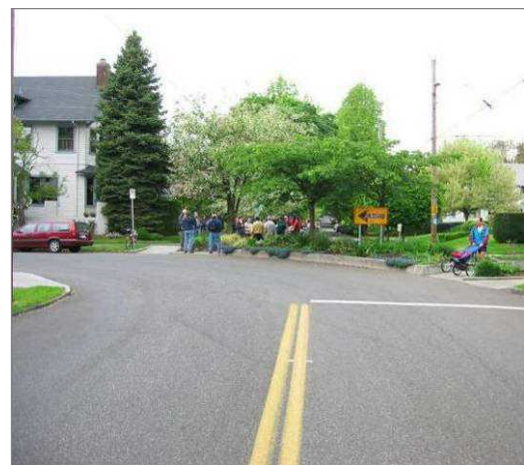
Traffic diverters prevent access to both directions of motor vehicle traffic.
